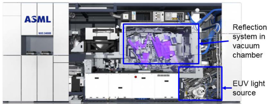
Figure 4.1.: Internal structure of ASML NXE:3400B scanner [18].
