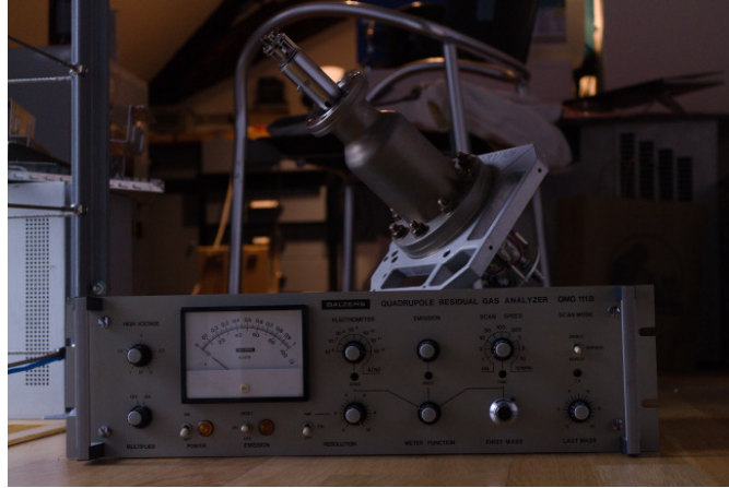
Figure 4.6.: Balzers quadrupole gas analyzer. Source: Sally Marcher
