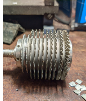
Figure 2.11.: Broken (left part) TMP rotor. Source: Sally Marcher
