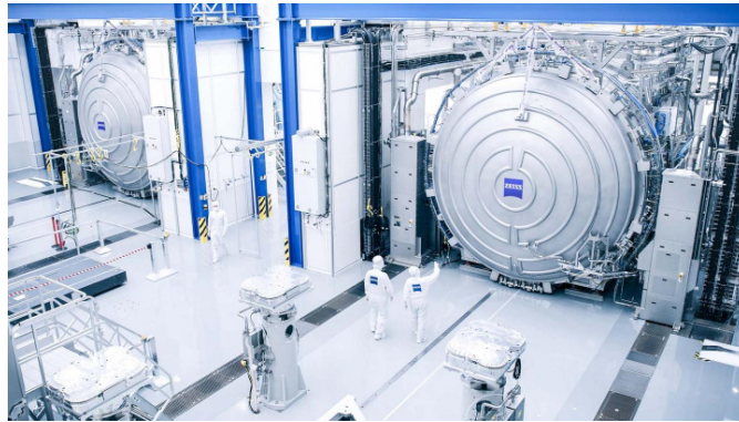
Figure 4.2.: Mirror testing facility from ZEISS with vacuum chambers measuring a diameter of five meters [29].
