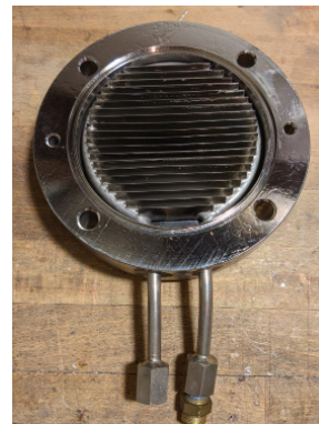
Figure 2.8.: Diffusion Pump Baffle. Source: Sally Marcher
