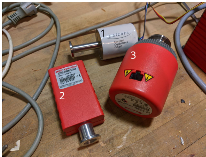
Figure 3.1.: Different vacuum sensors. Source: Sally Marcher
