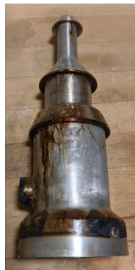
Figure 2.7.: Diffusion Pump stack. Source: Sally Marcher
