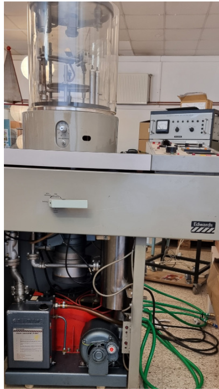
Figure 4.7.: Edwards E306 vacuum evaporation setup. Source: Ernst Pölzler
