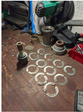
Figure 2.10.: Disassembled TMP. Source: Sally Marcher
